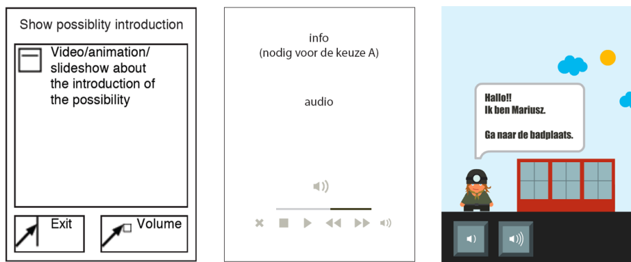
Fig. 5. Three levels of prototypes for one specific screen. From left to right: a Canonical Abstract prototype, a low-fidelity prototype and a high-fidelity prototype.
